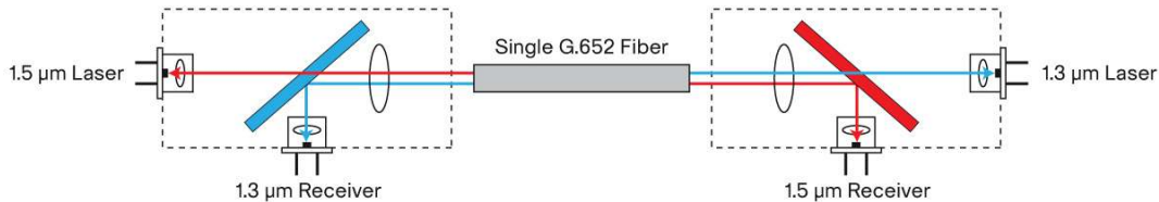
Figure 2. Bidirectional Transmission on a Single Strand of SMF
